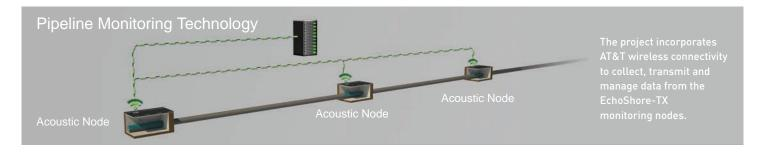
New pipeline monitoring technology combined with wireless communications and data visualization as demonstrated in the NIST Global City Teams Challenge are enabling utilities to ensure sustainability of their water system.
